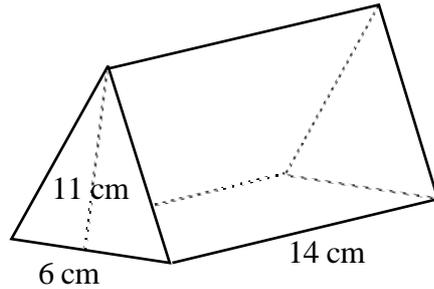
$$\text{Area}_{\text{end face}} = \frac{1}{2} b \times h$$
