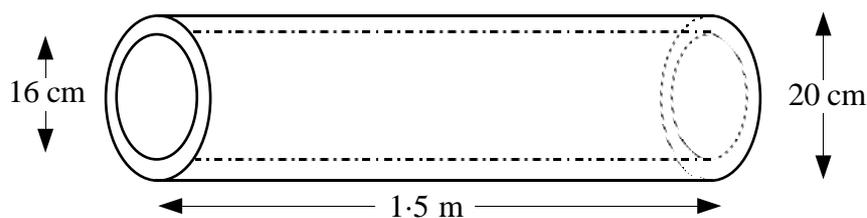
Calculate the volume of iron needed to make the pipe.
